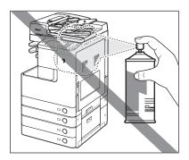
■ Do not use flammable sprays, such as spray glue near the machine. There is a danger of ignition.
